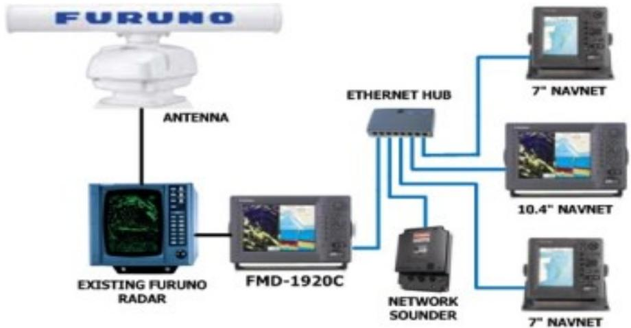
Note that changing the gain, STC or FTC on the master Furuno radars with Linear IF amplifiers (designated by a † symbol above) will affect the radar picture of the FMD-1920C. Additionally, Furuno radars with an \* require the optional buffer PCB, P/N 008-471-070. (This PCB is No longer available from Furuno USA)
